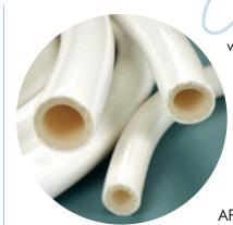
ffered as an alternative to mandrel-built wrapped silicone hose, APSH-DB provides several advantages over wrapped hose. APSH-DB, an extruded product, is less costly than wrapped hose and is available in lengths up to 50 feet. It offers more flexibility and comparable working pressure ratings. APSH-DB meets USP Class VI, FDA CFR 177.2600, ISO 10993, European Pharmacopoeia 3.1.9, and 3A standards.
